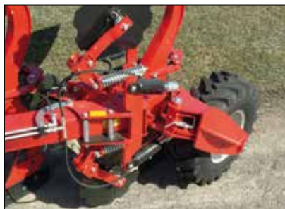
Hydraulic depth control and tractor treaded tire for combi wheel above.
