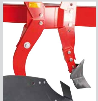
Shear Bolt: 16 mm 10.9 bolt quality, burst at a force of 4.000 kg
